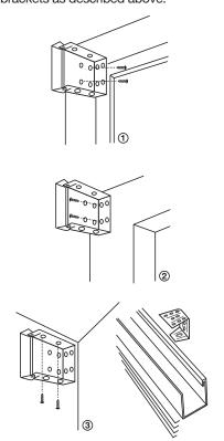
Step 4. Inserting the Head Rail
