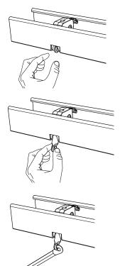
**Step 6.** Install Valance Clips and Valance For inside mounts - attach the clips to the valance as shown – position them evenly across the valance – before attaching the valance to the head rail be sure that the clips will not interfere with the mechanisms inside
