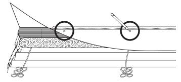
2. Using the pencil marks from Step 1 as center points, pencil mark 1-1/2" wide lines where the fabric meets the bottom edge of the head rail. Pierce the fabric at one end of each line with a utility knife, and slit the fabric for the entire length of the line – a sawing motion with the knife works best.
