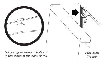
Inside Mount – lift the front of the shade to attach the set-screws.
